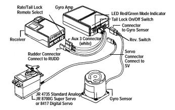
Step 3: On the amplifier, locate the SV (Servo) receptacle. Plug the rudder servo into this receptacle, noting the correct polarity as indicated by the shape of the plug, as well as the wire color.
