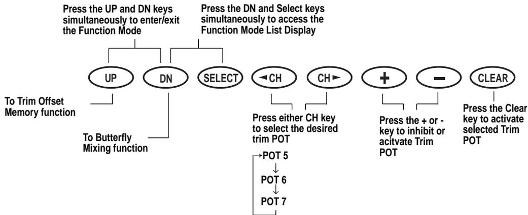
**Note:** Only POT 5 will appear on the LCD unless the Dual Flap Mixing Function is activated in the Wing Mixing Function. Refer to the Wing Mixing Function for more information on how to activate the Dual Flap Mixing Function.
