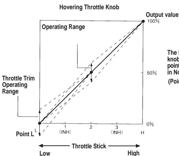
The hovering throttle knob adjusts all middle points that are activated in Normal Mode (Points 1 and 3)
