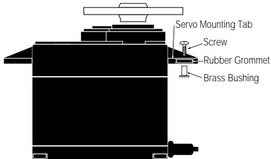
2. The servos should be mounted using rubber grommets and brass bushings to isolate them from vibration. Do not over-tighten the mounting screws — this will negate the vibration absorption effect of the rubber grommets. The diagram at left will assist you in properly mounting your servo.
