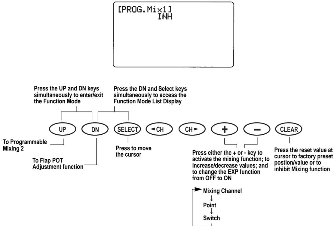
The XP8103 offers six (6) programmable mixes to be used for a number of different purposes. The functions allows mixing any one channel to any other channel.
