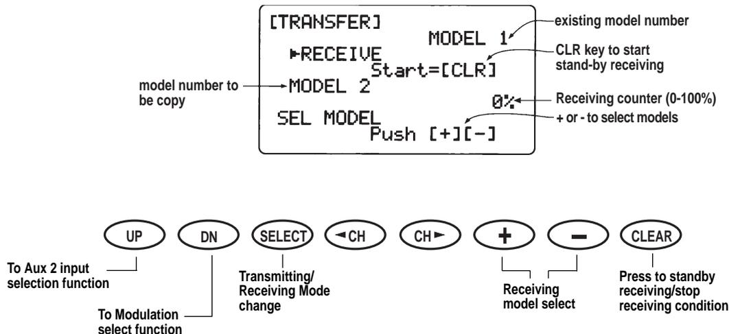
When the receiving counter is stopped or you see ERROR indicated, check the DSC cord connections or trainer cord conditions and try again. When data has been received correctly, you will see [End ok] display. Be sure that the receiving mode transmitter is in stand-by condition first. Then on the transmitting transmitter press the CLR key to start transmitting.
