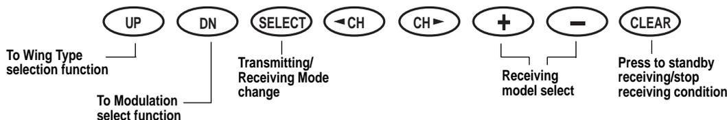
When the receiving counter is stopped or you see ERROR indicated, check the DSC cord connections or trainer cord conditions and try again. When data has been received correctly, you will see [End ok!] display. Be sure that the receiving mode transmitter is in stand-by condition first. Then on the transmitting transmitter press the CLR key to start transmitting.
