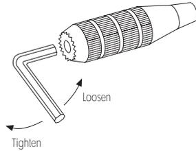
To adjust the stick length, use the 2 mm Allen wrench (supplied with your XP8103 transmitter) to unlock the set screw.
