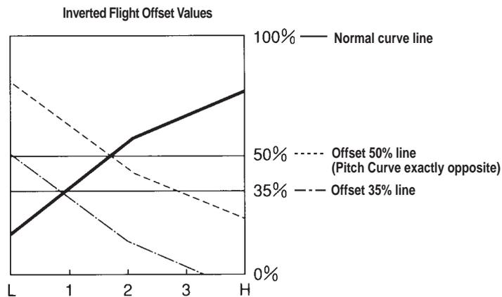
As shown above, when the offset value is set for 50%, the inverted flight pitch curve is exactly opposite from the normal pitch curve settings. If the offset is adjusted to a lesser value, say
