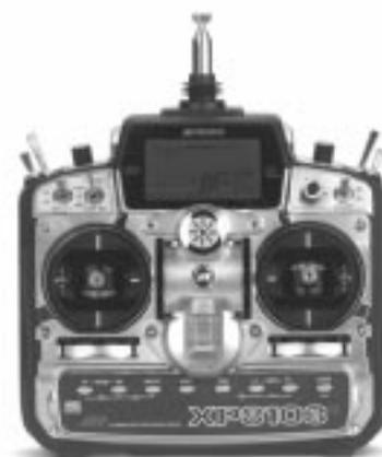
8 CHANNELS    10 MODEL MEMORY    3 MODEL TYPE    S • Z PCM/PPM SELECTABLE
