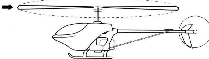
(3) When both blades are in track, the blade tips will appear to overlap as seen from the edge of the rotor plane.
