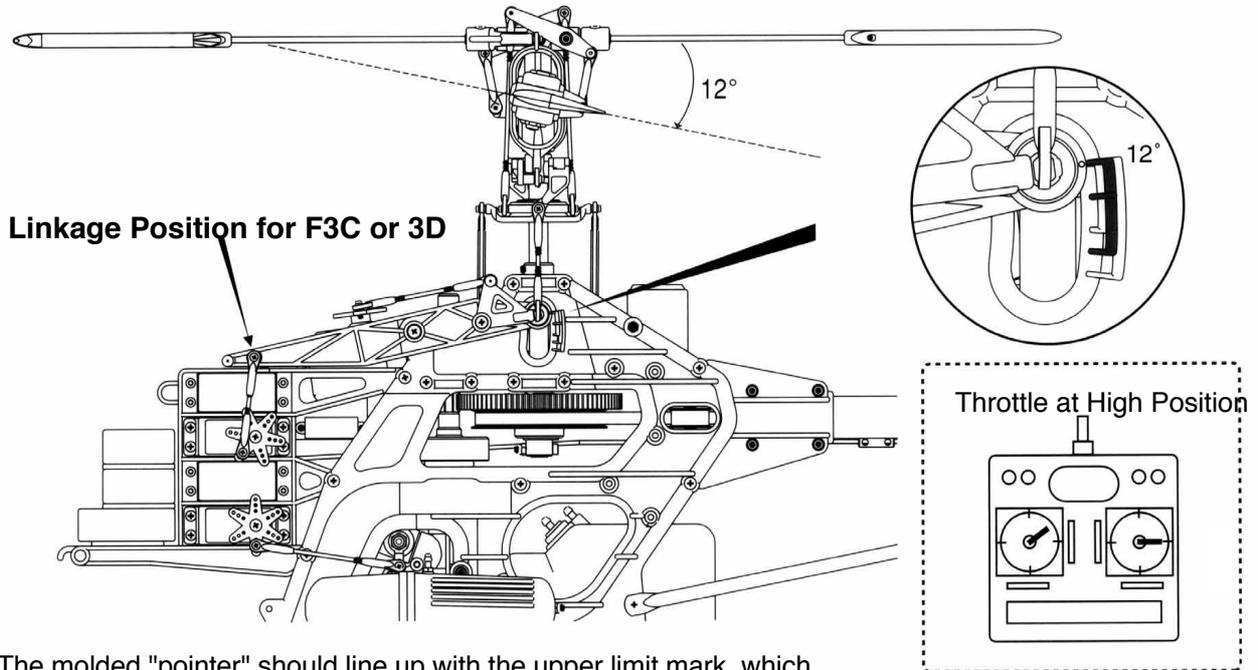
The molded "pointer" should line up with the upper limit mark, which should provide about 12° of blade pitch.
