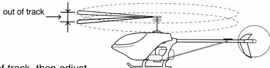
If the blades are out of track, then adjust one of the pushrods that connects to the main rotor blade pitch arm.
