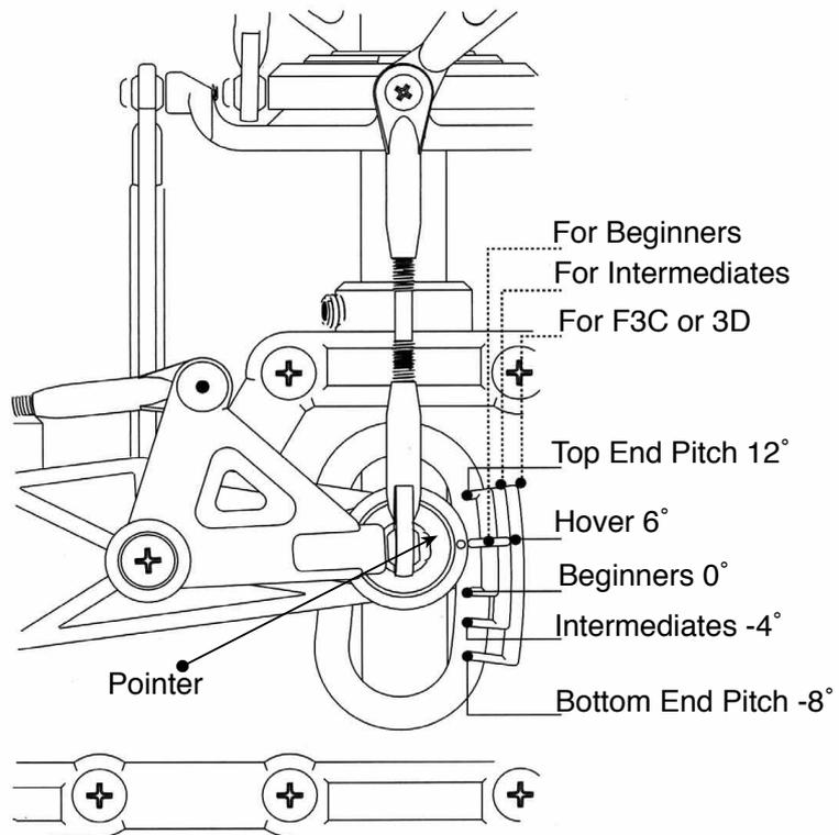
The hovering pitch angle should be at 6°. To get the 0° to 12° collective range, mount the steel linkage ball at 10.5mm away from the center of the collective servo horn.
