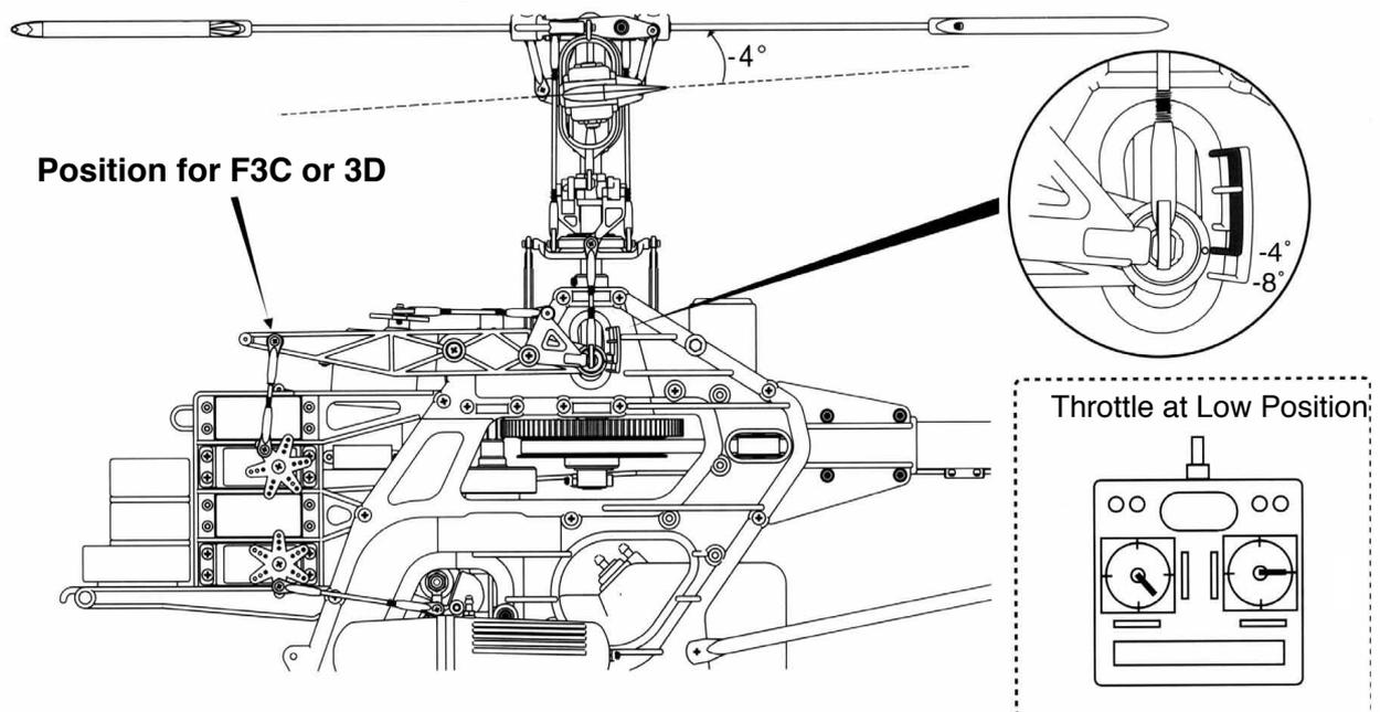
For intermediates set the low end to -4°. For advanced F3C and 3D flying, set the low end to -8°.
